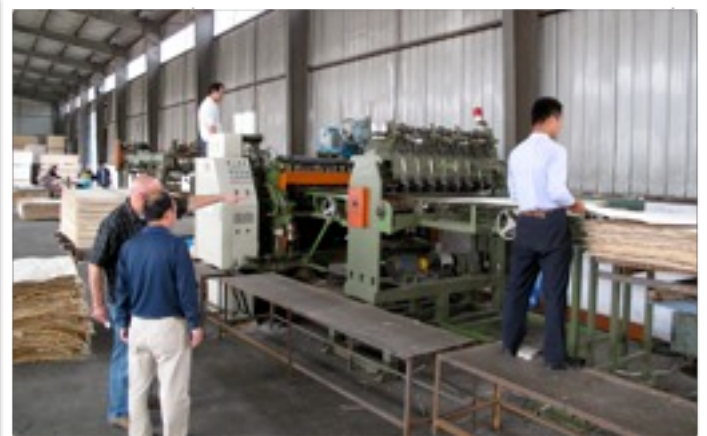
TigerPLY's Machine Core Composer used for C9 and TigerLITE Cores
